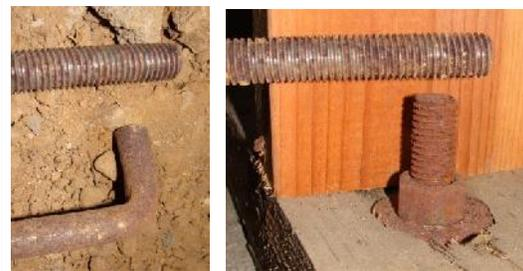
**Figure 8-52** Accidental experiment—the builder left a couple of foundation anchors lying on the dirt under a house (photo above left). Photo above right compares one of them to an anchor installed in PT lumber nearby. The anchor that had been left on the bare ground still has shiny portions, whereas rust completely covers the anchor installed in the PT lumber.
