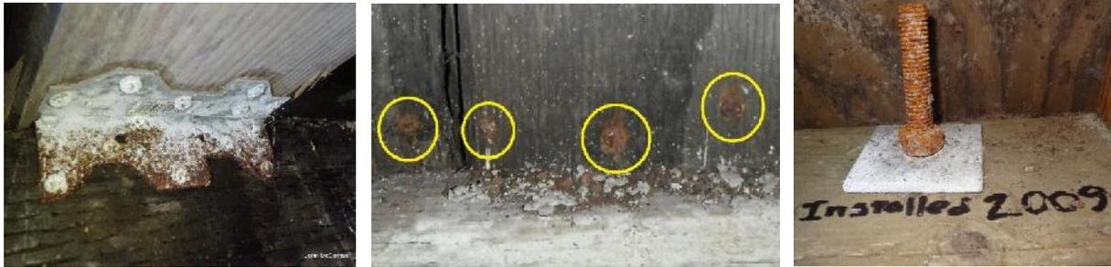
**Figure 8-47** Photos show severe corrosion that occurred within five years of construction. *Left: “White rust” turning to red rust. Photo: John McComas, GGASHI* *Center: Remains of nails used to fasten PT plywood. Photo: Keith Tarkington, GGASHI* *Right: Mudsill anchor photographed by author in May, 2014.*
